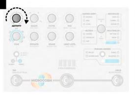
(2) In Global Configuration mode, each control knob is assigned to a specific configuration menu. You can access these options by turning any one of the assigned knobs and opening the color-coded menu (In the example for steps 2 & 3, the Activity knob is being used to access the "input mode" configurations).
