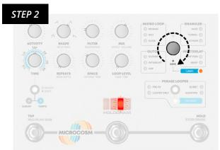
(2) Cursor will blink to indicate copied material. Turn to the desired **User Preset** slot and hold down the Selector again to save the preset.
